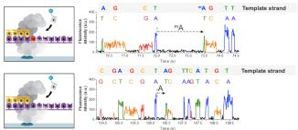
The presence of a modified base (6-mA) in the template (top) causes a delayed incorporation of the corresponding T nucleotide (longer IPD) compared to a control DNA template lacking modification (bottom).
