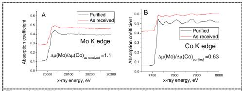
**Figure 4.** XANES data in the as-received and purified nanotubes measured at (a) Mo K-edge and (b) Co K- edge. The edge step ratio (Mo:Co) decreases after purification.
