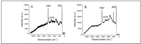
**Figure 1.** Raman spectra of (a) as-received SWNTs and (b) purified SWNTs. The peak at 518 cm<sup>-1</sup> is due to the Si wafer used to support the purified powder.
