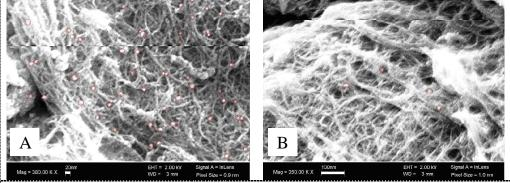
**Figure 2.** SWNTs (a) before and (b) after purification. Red rings around nanoparticles have been added for clarity. The scale bars are 20 nm (a) and 100 nm (b) in lengths.
