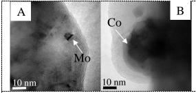
**Figure 3.** TEM images showing (a) Mo-rich and (b) Co-rich particles
