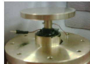
Figure 5: Wire connections on bottom plate
