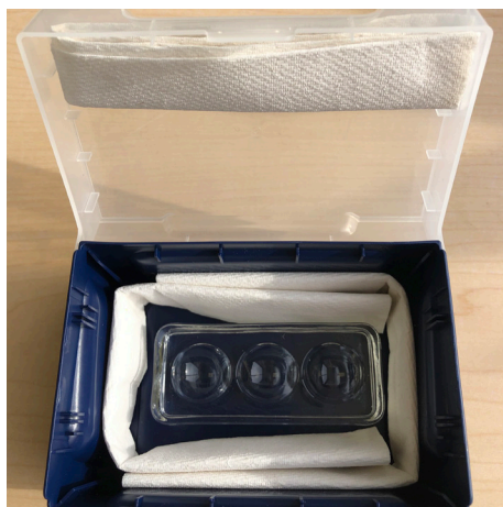
Figure 2. An in-house humidity incubation box. Wet paper towels are placed along the four bottom edges of an empty pipette box and dry paper towel is attached to the inner surface of the lid. The wet paper towels should create a pocket for a spot plate to fit in.
