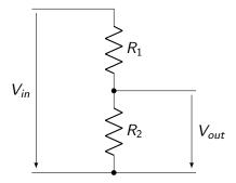
What is  $V_{out}$  as function of  $V_{in}$ ?
