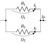
KVL: Voltage across both resistors is the same:  $U_1 = U_2 = U$ Total current is the sum:  $I_p = I_1 + I_2 = U/R_1 + U/R_2$
