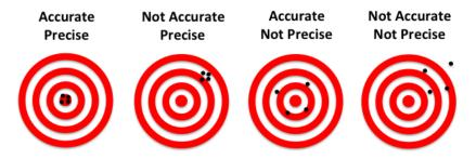
Measure a mass with a scale Precision ( $\sim$ statistical error):
