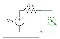
• We can get the voltage by measuring the unloaded voltage. No current flows, so there is no drop over  $R_{Th}$ , so  $V_{\text{measured}} = V_{Th} = V$ (open circuit)
