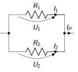
KVL: Voltage across both resistors is the same:  $U_1 = U_2 = U$ Total current is the sum:  $I_p = I_1 + I_2 = U/R_1 + U/R_2$ Equivalent resistance is  $R_{eq} = U/I_P = \frac{1}{1/R_1 + 1/R_2}$ Or:  $G_p = G_1 + G_2$
