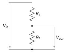
What is  $V_{out}$  as function of  $V_{in}$ ? Series resistance:  $I = V_{in}/(R_1 + R_2)$ Ohms law:  $V_{out} = R_2 I = V_{in} \frac{R_2}{R_1 + R_2}$
