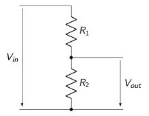
What is  $V_{out}$  as function of  $V_{in}$ ? Series resistance:  $I = V_{in}/(R_1 + R_2)$
