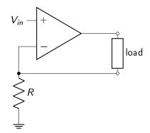
GRs:  $V_- = V_+ = V_{in}$
