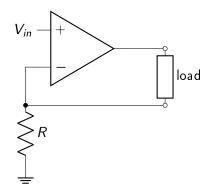
GRs:  $V_- = V_+ = V_{in}$
