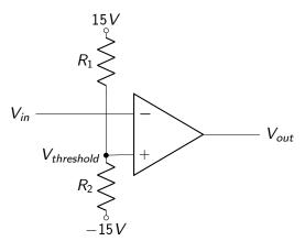
For  $V_{in} \neq V_{Threshold}$ , the output will saturate at it's minimum or maximum. Optimized opamps for this purpose exist, they are called comparators. Simplest form of an analog to digital converter!
