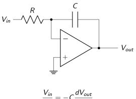
$$V_{out}(t) = rac{1}{RC}\int V_{in}(t) + {
