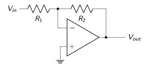
V<sub>+</sub> = 0V, so V<sub>-</sub> = 0V (This is called a virtual ground.)
