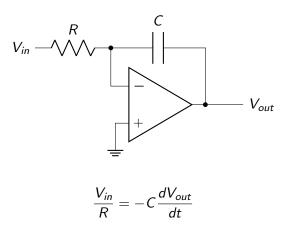
$$V_{out}(t) = rac{1}{RC}\int V_{in}(t) + {
