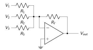
$$\frac{V_1}{R_1} + \frac{V_2}{R_2} + \frac{V_3}{R_3} + \frac{V_{out}}{R_f} = 0$$
