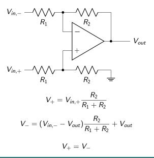
$$(V_{in,-} - V_{out}) \frac{R_2}{R_1 + R_2} + V_{out} = V_{in,+} \frac{R_2}{R_1 + R_2}$$
