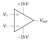
In circuit diagrams, the positive rail is often named  $V_{CC}$ , the negative  $V_{EE}$ DANGER: Sometimes, they are also named  $V_+$  and  $V_-$
