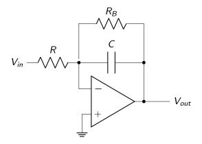
We want to make  $R_B$  very, very large. These resistors are hard to come by and have bad parasitic parameters (mainly capacitance)
