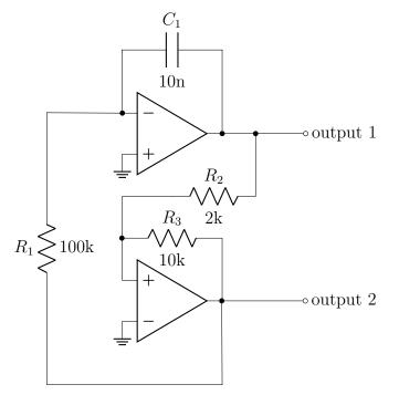
Using the two opamps in a single TL082, build the circuit. Do you observe the expected behavior?
