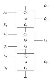
• Slowest path is carry, which has to ripple through all FAs. Other name: Ripple carry adder RCA In addition to fixed function ICs, there exists programmable logic. The most capable version of this are called FPGA: Field Programmable Gate Arrays
