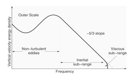
Large eddies dominate the production of TKE, the size of eddies decreases in the inertial sub-range until the length scales are small enough for molecular diffusion to dissipate kinetic energy into heat in the viscous sub-range
