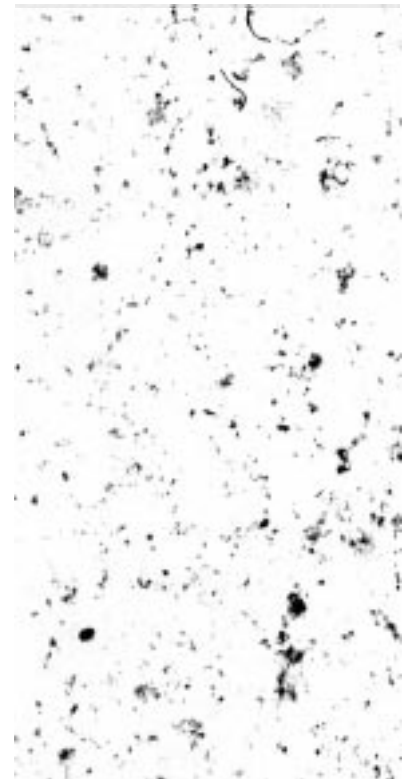
Figure 2. One to one magnified light absorption image of large particles captured by in-situ filtration at 200m in the Slope Water of the NW Atlantic. Particles shown are dominant contributors to vertical carbon flux and represent the catch from several cubic meters of seawater.
