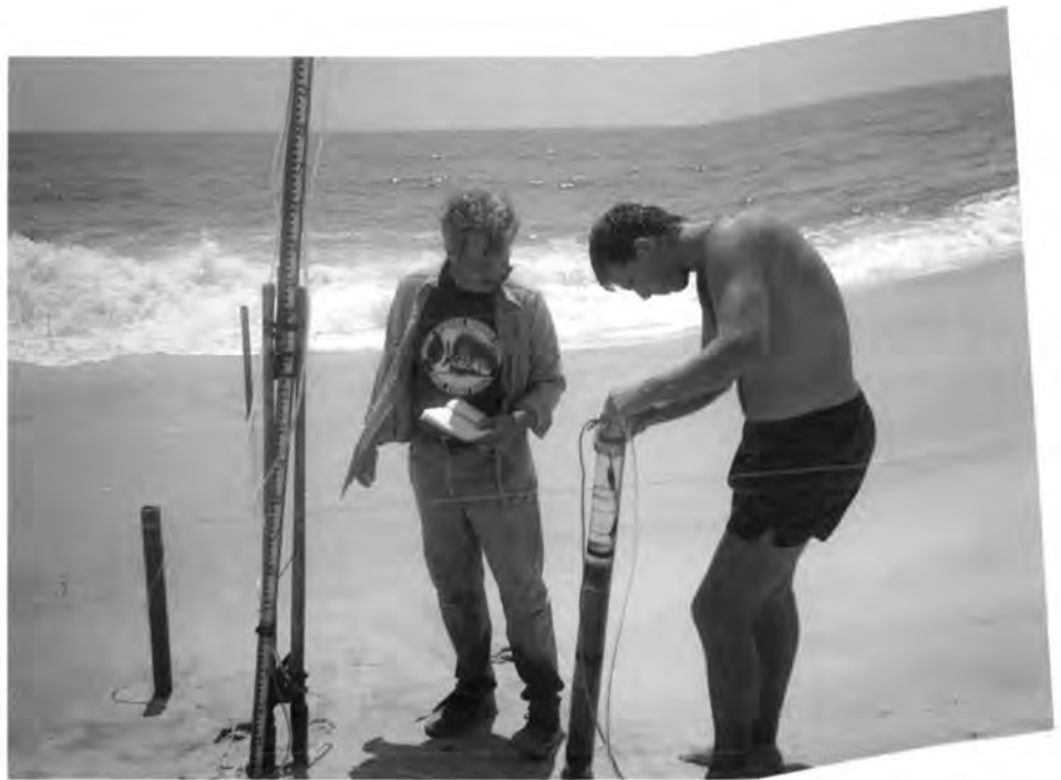
▲ Professor Henry Bokuniewicz and graduate student Chris Schubert look for changes in the beach by measuring water table elevations.
