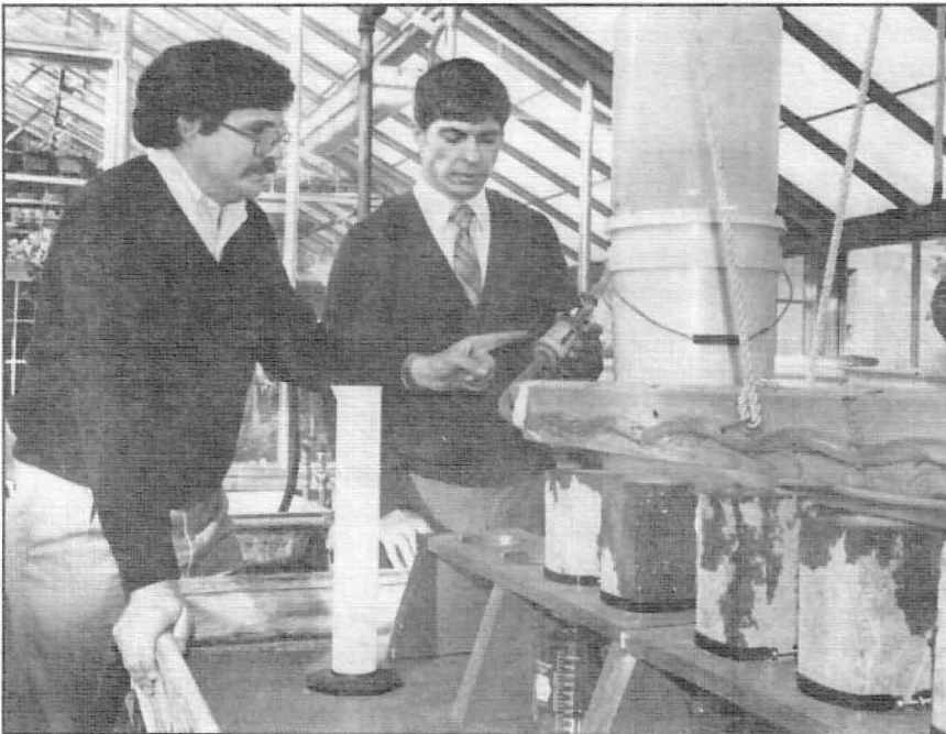
Dr. James M. Hassett, left, and Richard McClimans test construction blocks made from incinerator ash.
