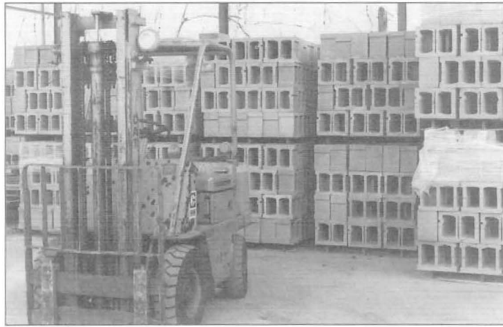
Figure 3: Incinerator residue blocks stacked ready for use in boat-house construction at the Marine Sciences Research Center, State University of New York at Stony Brook
